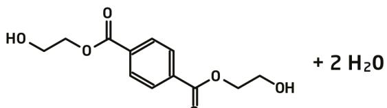
AN EXAMPLE OF POLYESTER BY STEP-GROWTH POLYMERIZATION UN ESEMPIO DI POLIESTERE PER POLICONDENSAZIONE
